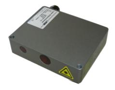
The sensors from the LASE 1000T Grey-Line Series are contactless one-dimensional distance meters especially built for the operation in harsh industrial environments.
